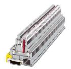
Component terminal block, nom. voltage: 500 V, nominal current: 34 A, 1st and 2nd level, connection method: Screw connection, Rated cross section:  $4 \text{ mm}^2$ , cross section:  $0.2 \text{ mm}^2$  -  $4 \text{ mm}^2$ , mounting: NS 35/7.5, NS 35/15, color: gray
