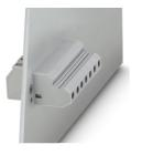
Panel feed-through terminal block, connection method: Screw connection with tension sleeve, Screw connection with tension sleeve, number of positions: 1, load current: 32 A, cross section:  $0.2 \text{ mm}^2 - 6 \text{ mm}^2$ , connection direction of the conductor to plug-in direction: -90 °, width: 8.1 mm
