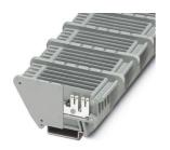
Feed-through terminal block, nom. voltage: 800 V, nominal current: 30 A, number of connections: 10, number of positions: 1, connection method: Spade connection, 1 level, cross section:  $0.5 \text{ mm}^2$  - 6 mm<sup>2</sup>, mounting type: NS 35/7,5, NS 35/15, color: gray
