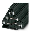
Multi-level terminal block, nom. voltage: 500 V, nominal current: 19 A, connection method: Screw connection, Rated cross section: 2.5 mm<sup>2</sup>, cross section: 0.14 mm<sup>2</sup> - 4 mm<sup>2</sup>, mounting type: NS 35/7,5, NS 35/15, color: black
