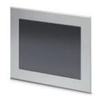
Rugged touch panel with 38.1 cm / 15" TFT display (analog-resistive (GFG)), 1024 x 768 pixels (XGA), degree of protection: IP67 (front), extended temperature range, ARM® Cortex® A8, 1000 MHz, Windows® Embedded Compact 7 and Visu+ application software.
