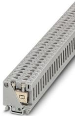
Mini feed-through terminal block, nom. voltage: 500 V, nominal current: 17.5 A, number of connections: 2, connection method: Screw connection, 1 level, Rated cross section: 1.5 mm<sup>2</sup>, cross section: 0.2 mm<sup>2</sup> - 2.5 mm<sup>2</sup>, mounting type: NS 15, color: gray
