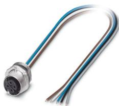
Device connector front mounting, Universal, 5-position, Socket, straight, M12-SPEEDCON, coding: A, on free cable end, Front mounting, M16 x 1.5, Individual wires, cable length: 1 m, 0.34 mm<sup>2</sup>, TPE litz wire
