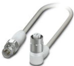
Sensor/actuator cable, 4-position, PP-EPDM halogen-free, gray RAL 7035, Plug straight M12, A-coded, on Socket angled M12, A-coded, with 3 LEDs, cable length: 0.6 m, Hygienic design, with high-grade steel knurl
