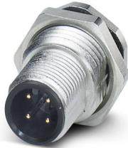
Device connector rear mounting, 4-position, Pin, straight, M12, coding: A, Rear mounting, Pg9, Wave soldering, Alternative product in accordance with RoHS II without Exemption 6c (Pb < 0.1 %) item no.: 1238709
