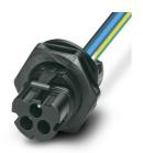
Device connector, rear mounting, Range of articles: PRC 35, housing material: PPE, color: black, number of positions: 3, max. conductor cross section: 6 mm², rated voltage: 690 V AC, rated current: 35 A, Connection method: Crimp connection, Contact connection type: Pin, cable length: 150. This item is also available with other cable lengths. For your specific requirements, please contact your local PHOENIX CONTACT subsidiary.
