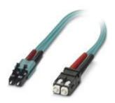
Assembled FO cable, zip cord cable, multi-mode fiberglass 50/125  $\mu$ m, OM3, plug: LC/SC-RJ, degree of protection: IP20, for installation in cable ducts or control cabinets, length: 1 m
