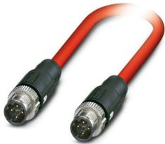
Network cable, Sercos CAT5 (100 Mbps), 4-position, PVC/PVC, signal red RAL 3020, shielded, Plug straight M12 SPEEDCON, coding: D / IP67, on Plug straight M12 SPEEDCON, coding: D / IP67, cable length: 10 m
