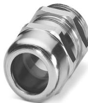
Cable gland, material for screw connection: Brass, nickel-plated, application: Standard, external cable diameter 13 mm ... 18 mm, shielding: no, connecting thread: Pg21, color: silver, with O-ring
