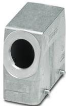
Sleeve housing B24, for double locking latch, material: Die-cast aluminum, salt water resistant, cable outlets: 1, lateral, 1x Pg21, height: 76 mm, cable gland: none, Standard
