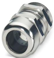
Cable gland, material for screw connection: Brass, nickel-plated, application: EMC, external cable diameter 13 mm ... 18 mm, shielding: yes, connecting thread: Pg21, color: silver, with O-ring
