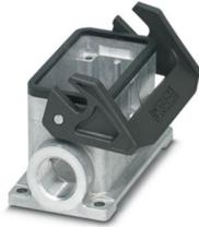
Box mounting bases B10, with single locking latch, material: Die-cast aluminum, salt water resistant, cable outlets: 2, lateral, 2x M25, height: 54.6 mm, cable gland: none, Standard
