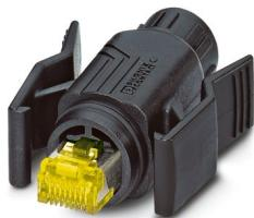
RJ45 connector, design: RJ45, degree of protection: IP67, number of positions: 8, 10 Gbps, CAT6<sub>A</sub>, material: Plastic, connection method: Crimp connection, connection cross section: AWG 24- 27, cable outlet: straight, color: black, Ethernet/PROFINET
