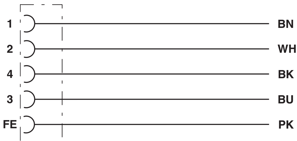
Contact assignment of the M12 socket
