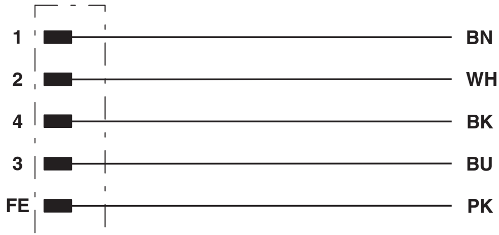
Contact assignment of the M12 plug
