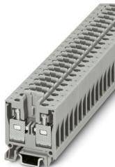
Disconnect terminal block, Current and voltage are determined by the plug used., nom. voltage: 500 V, nominal current: 16 A, connection method: Screw connection, Rated cross section: 4 mm<sup>2</sup>, cross section: 0.2 mm<sup>2</sup> - 4 mm<sup>2</sup>, mounting: NS 15, color: gray
