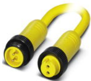
Power cable, 2-position, PVC, yellow, Plug straight 7/8"-16UNF, A - standard, on Socket straight 7/8"-16UNF, cable length: 2 m
