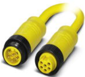
Power cable, 6-position, PVC, yellow, Plug straight 7/8"-16UNF, A - standard, on Socket straight 7/8"-16UNF, A - standard, cable length: 2 m
