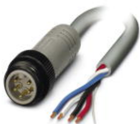
Bus system cable, DeviceNet™, 5-position, PVC, gray, Plug straight 7/8"-16UNF, A - standard, on free cable end, A - standard, cable length: 5 m
