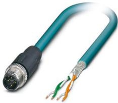
Network cable, Ethernet CAT5 (100 Mbps), 4-position, PUR halogen-free, water blue RAL 5021, shielded (Aluminum-coated foil, tinned copper braided shield), Plug straight M12, coding: D / IP67, on free cable end, cable length: 15 m
