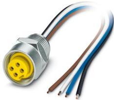
Flush-type connector, 4-position, Socket, straight, 7/8"-16UNF, on free cable end, Front mounting, with 1/2 inch-14 NPT mounting thread, Individual wires, cable length: 1 m, 0.75 mm<sup>2</sup>, PVC litz wire
