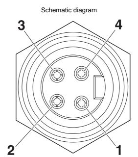
Pin assignment, socket, 7/8"-16UNF, 4-pos., view of female side (reference image)
