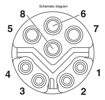
Pin assignment M12 socket, 8-pos.
