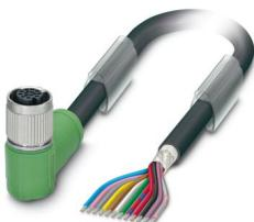
Sensor/actuator cable, 12-position, PUR/PVC, black RAL 9005, shielded (Tinned copper braided shield), free cable end, on Socket angled M12 SPEEDCON, coding: A, cable length: 5 m
