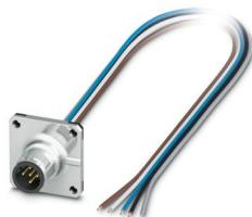
Device connector front mounting, 5-position, Pin, straight, M12, coding: B, on free cable end, Front mounting, Square flange, Individual wires, cable length: 0.5 m, 0.34 mm<sup>2</sup>, TPE litz wire, Alternative product in accordance with RoHS II without Exemption 6c (Pb < 0.1 %) item no.: 1239718
