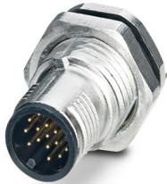
Device connector rear mounting, 17-position, Pin, straight, M12, coding: A, Rear mounting, M16 x 1.5, Solder pins, Alternative product in accordance with RoHS II without Exemption 6c (Pb < 0.1 %) item no.: 1239755
