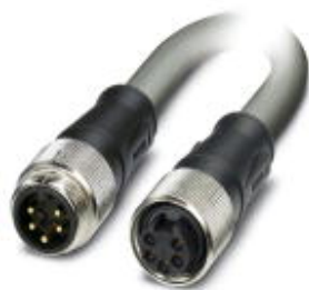
Power cable, 5-position, PVC, Gray RAL 7001, Plug straight 7/8"-16UNF, A-coded, on Socket straight 7/8"-16UNF, A-coded, Cable length: 0.3 m, 2.5 mm 2 conductor cross section, For power supply
