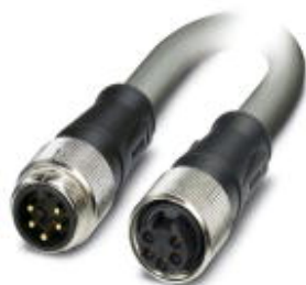
Power cable, 5-position, PVC, Gray RAL 7001, Plug straight 7/8"-16UNF, A-coded, on Socket straight 7/8"-16UNF, A-coded, Cable length: 2 m, 2.5 mm 2 conductor cross section, For power supply
