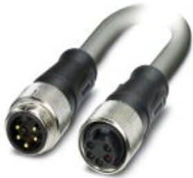
Power cable, 5-position, PUR, gray RAL 7001, Plug straight 7/8"-16UNF, A-coded, on Socket straight 7/8"-16UNF, A-coded, cable length: 1.5 m, 1.5 mm 2 conductor cross section, For power supply
