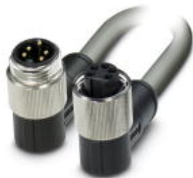
Power cable, 5-position, PUR, gray RAL 7001, Plug angled 7/8"-16UNF, on Socket angled 7/8"-16UNF, cable length: 1.5 m, 1.5 mm 2 conductor cross section, For power supply
