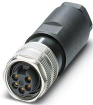
Connector, Universal, 5-position, Socket straight 7/8"-16UNF, coding: A, Screw connection, knurl material: Zinc die-cast, nickel-plated, cable gland Pg13,5, external cable diameter 10 mm ... 12 mm
