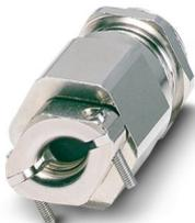
Cable gland, material for screw connection: Brass, nickel-plated, application: Standard, external cable diameter 6 mm ... 13 mm, shielding: no, connecting thread: M20 x 1.5, color: silver, with external strain relief, with O-ring
