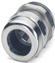
Cable gland, material for screw connection: Brass, nickel-plated, application: EMC, external cable diameter 9 mm ... 13 mm, shielding: yes, connecting thread: M20 x 1.5, color: silver, with O-ring
