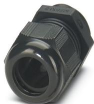
Cable gland, material for screw connection: PA, application: Standard, external cable diameter 6 mm ... 12 mm, shielding: no, connecting thread: M20 x 1.5, color: jet black RAL 9005
