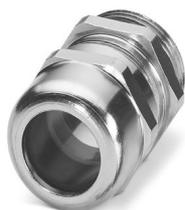
Cable gland, material for screw connection: Brass, nickel-plated, application: Standard, external cable diameter 6 mm ... 12 mm, shielding: no, connecting thread: M20 x 1.5, color: silver, with O-ring
