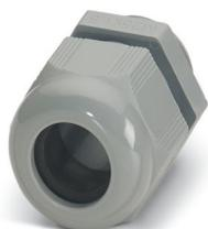
Cable gland, material for screw connection: PA, application: Standard, external cable diameter 6 mm ... 12 mm, shielding: no, connecting thread: M20 x 1.5, color: silver-grey RAL 7001
