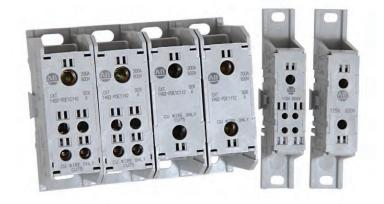
1492-PDME/PDE Enclosed Power Distribution Terminal Blocks are designed to prevent accidental contact with live connectors—without the use of additional barriers or shields. These panel mount devices have a compact footprint, and are available with either aluminum or copper terminals. Captive termination screws ensure that parts never get lost and the rugged thermoplastic housing will resist physical damage.
