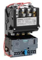
Non-reversing motor starter Size 0 Single phase full voltage Solid-state overload relay OLRelay amp range 5.5-22A 110-120/220-240VAC 60HZ coil Combination type No enclosure
