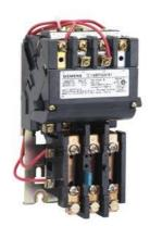
Non-reversing motor starter, Size 1, Single phase, 2-pole, Amb compensate bimetal OLrelay Contactor amp rating 27Amp 220 240/440 480VAC 60HZ coil, Non-combination type, Enclosure type (open), No enclosure
