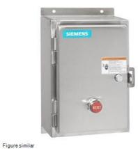
Non-reversing motor starter, Size 1, Single Phase, 2-Pole, Amb. compensate bimetal OLR, Contactor amp rating 27A, 110V 50Hz / 120V 60Hz coil, Non-combination type, Encl. type 4X 304 S. Steel, Water/dust tight noncorrosive
