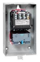
Non-reversing motor starter Size 1 Three phase full voltage Solid-state overload relay OLRelay amp range 0.25-1A 220-240/440-480VAC 60HZ coil Combination type Indoor general purpose use
