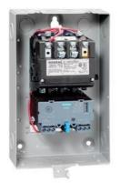
Non-reversing motor starter Size 1 Three phase full voltage Solid-state overload relay OLRelay amp range 0.25-1A 190-220/220-240V 50/60HZ coil Combination type Indoor general purpose use
