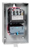
Non-reversing motor starter, Size 1, Single phase full voltage, Solid-state overload relay, OLR amp range 0.75-3.4A, 24VAC 50-60Hz coil, Non-combination type, Enclosure type 1, Indoor general purpose use, Standard width enclosure
