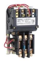
Non-reversing motor starter, Size 1 3/4, Single phase, 2-pole, Amb compensate bimetal OLrelay Contactor amp rating 40Amp 24VAC 50-60HZ coil, Noncombination type, Enclosure type (open), No enclosure
