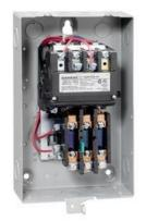
Non-reversing motor starter, Size 1 3/4, Single Phase, 2-Pole, Amb. compensate bimetal OLR, Contactor amp rating 40A, 208VAC 60Hz coil, Non-combination type, Enclosure type 1, Indoor general purpose use
