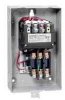
Non-reversing motor starter, Size 1 3/4, Single Phase, 2-Pole, Amb. compensate bimetal OLR, Contactor amp rating 40A, 24VAC 50-60Hz coil, Non-combination type, Enclosure type 1, Indoor general purpose use
