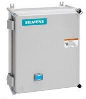
Non-reversing motor starter, Size 1 3/4, Single Phase, 2-Pole, Amb. compensate bimetal OLR, Contactor amp rating 40A, 110V 50Hz / 120V 60Hz coil, Non-combination type, Enclosure type 4X fiberglass, Water/dust tight noncorrosive
