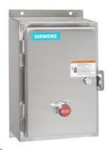
Non-reversing motor starter, Size 1 3/4, Single Phase, 2-Pole, Amb. compensate bimetal OLR, Contactor amp rating 40A, Non-combination type, Encl. type 4X 304 S. Steel, Water/dust tight noncorrosive
