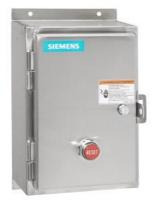
Non-reversing motor starter, Size 1 3/4, Single Phase, 2-Pole, Amb. compensate bimetal OLR, Contactor amp rating 40A, 110V 50Hz / 120V 60Hz coil, Non-combination type, Encl. type 4X 304 S. Steel, Water/dust tight noncorrosive
