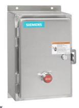
Non-reversing motor starter, Size 1 3/4, Single Phase, 2-Pole, Amb. compensate bimetal OLR, Contactor amp rating 40A, Non-combination type, Encl. type 4X 304 S. Steel, Water/dust tight noncorrosive
