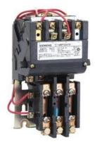
Non-reversing motor starter, Size 1 3/4, Three phase full voltage, Amb compensate bimetal OLrelay Contactor amp rating 40Amp 110V 50HZ / 120V 60HZ coil, Non-combination type, Enclosure type (open), No enclosure
